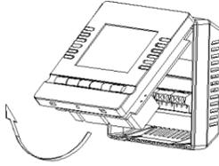
2. Take the main control panel apart: put the screwdriver (3.5mm wide) into 4mm of slot.
