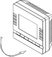
6. Push the downside by force, lock the up panel, and finish the installation.
